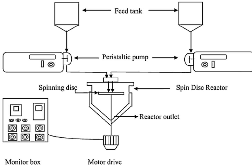
Figure 1. Basic design of a spinning disc reactor [2].
