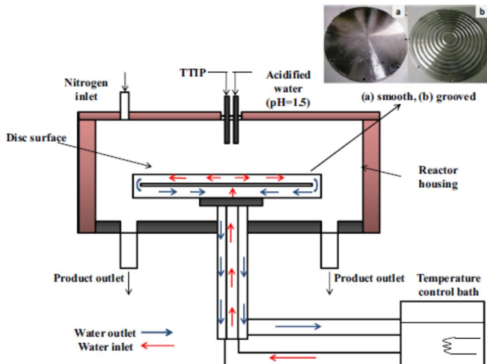
Figure 7. Experimental setup for the production of TiO<sub>2</sub> nanoparticles [3].
