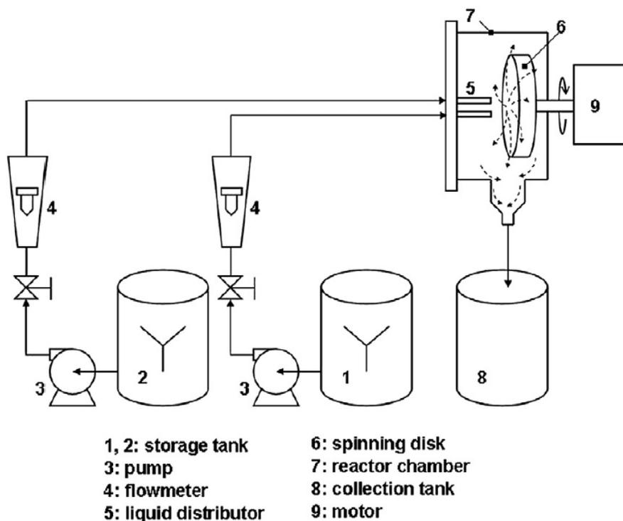
a vertical SDR as seen in Figure 4. The resulting compound was put through a calcination process to form the resulting copper oxide ( $\text{CuO}$ ) [6].
