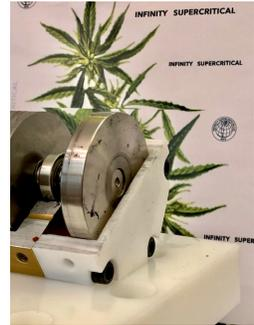
Magnetic couplings connect the drive motor to rotating assemblies through air.
